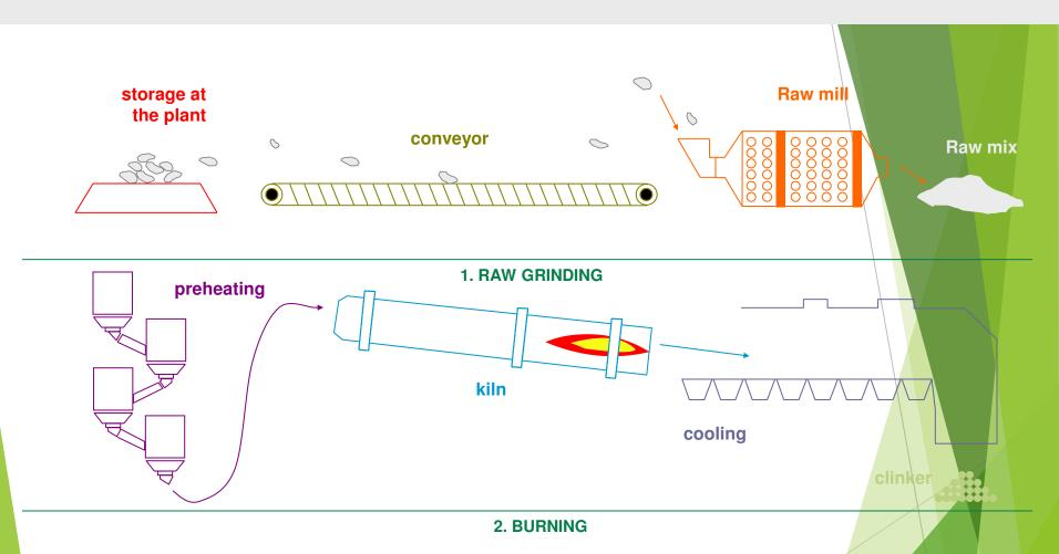
1. RAW GRINDING : The raw materials are very finely ground in order to produce the raw mix.
